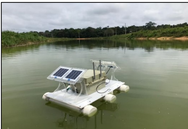
Figure 3. Image of the autonomous experimental station (AES) developed and tested in commercial fishponds in the state of Amazonas, Brazil
