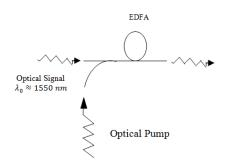
Figure 2. An erbium-doped fiber amplifier
