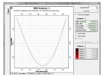
Figure 9 min. BER at fibre length 10 of 16 users WDM (40 Gbps)
