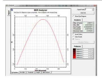
Figure 7 Min. BER of 40 Gbps WDM system with 16 users
