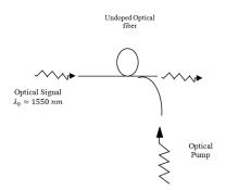
Figure 4. A fiber Raman optical amplifier
