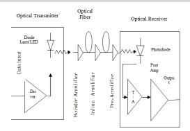
Figure 1. Optical amplifiers in a fiber optic data link
