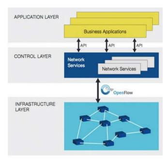
Fig. 1. Software Defined Networking (SDN) Framework
